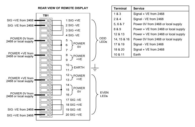
Figure 4.6 - Cable connection details for the remote display
